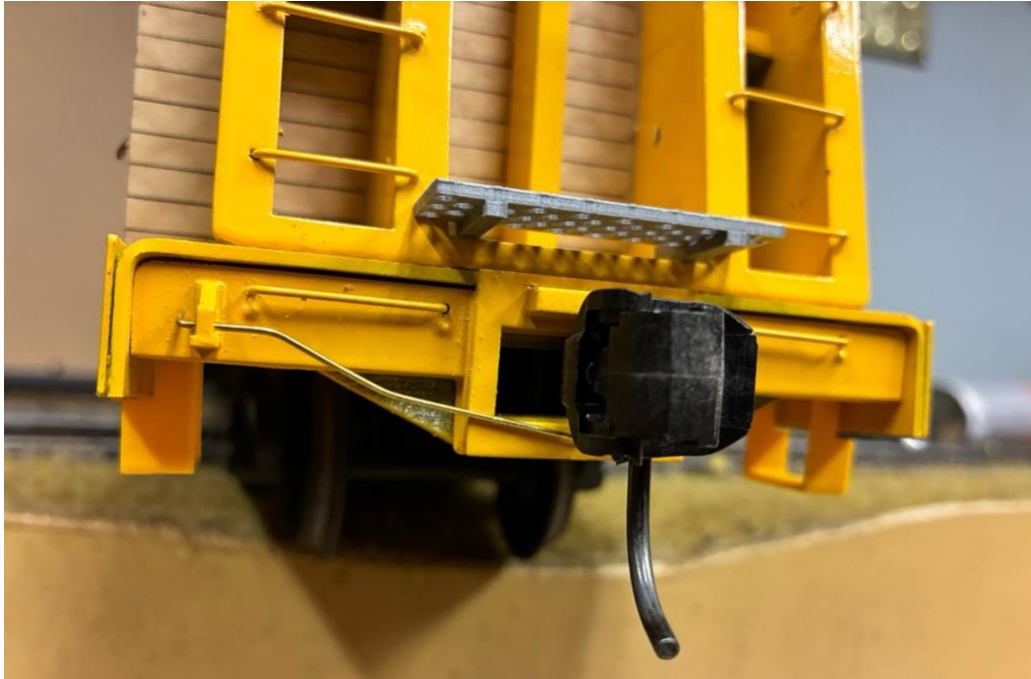
PHOTO 8: Cut Lever Detail Photo
