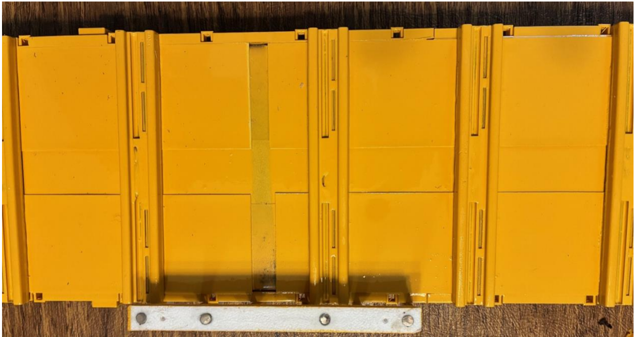
PHOTO 15 Underside of Finger Rack showing Magnets (White) and Space on Deck where Finger Racks are to be located
