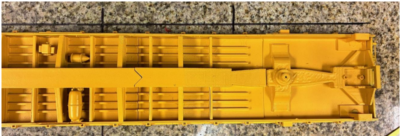
PHOTOS 9 & 10: Underside of F68 Flatcar Showing Brake Component Locations
