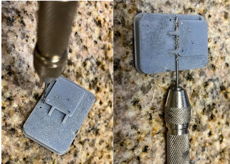
PHOTO 5, 6 & 7: Grab Iron Bending Fixture
